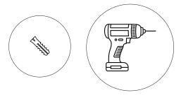
2 Now let's drill some pilot holes over the marked-out hole locations. A 4mm drill bit will do the job when screwing straight into a wall stud. If using the plastic anchor supplied, drill a 6-7mm hole. When installing the anchors, you may need to lightly tap them in with a hammer. We recommend using the plastic anchors supplied when positioned over plasterboard. Concrete walls will require their own screw anchor specifically designed for concrete.
